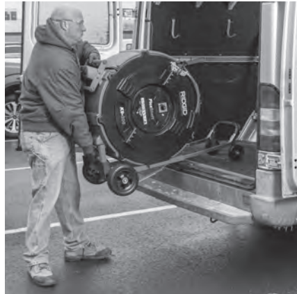
Figure 17 – Lifting Unit Onto Vehicle
